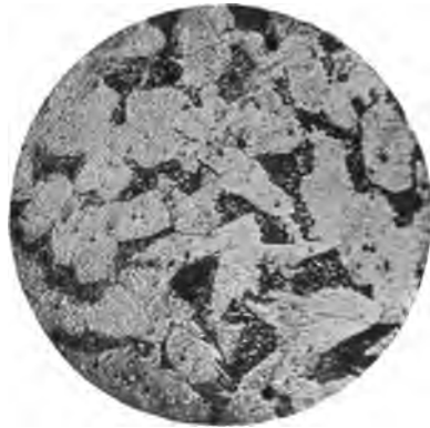
FIG. 68.—Mild Steel (Preuss) cooled slowly. Ferrite and Pearlite ( \times 350 ).
